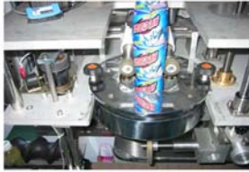
切刀座 UNIQUE BLADE SEAT 特殊设计的钢体结构，采用自旋式静态裁切，免用碳刷，裁切精准均一。 Special design with steel constructs. Static self-rotating cutting guarantee the precise cutting and no carbon brush will be used
